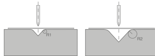
V-bending with narrow and wide dies
