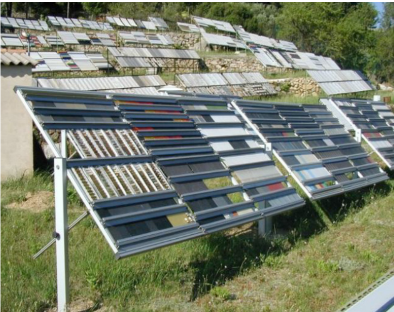
Granite ® HDX test panels at the Station d'Essais de Vieillessement Naturel (SEVN) in Sanary-sur-Mer, France. Photograph: © ArcelorMittal Global R&D
